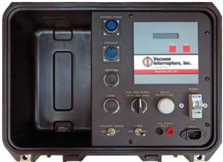
CBT-1201 captures and stores trip, close, and bounce times in milliseconds.
